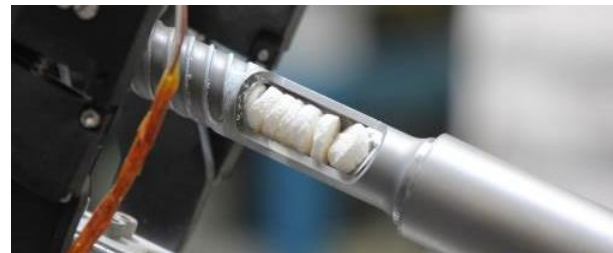
Figure 5. The PreView bit allows capture and in-situ analysis of rock cores.
